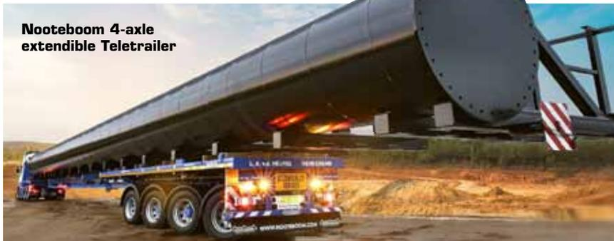
**Nooteboom 4-axle extendible Teletrailer**
