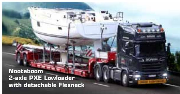
**Nooteboom 2-axle PXE Lowloader with detachable Flexneck**
